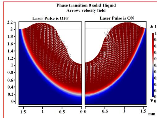
*Phase distribution and spatial velocity field (Left: when laser pulse is OFF cooling occurs and only marangoni convection and gravitational force is effective, Right: When laser pulse is ON recoil pressure acts and splashes the molten metal as shown by the arrow plot.).*
